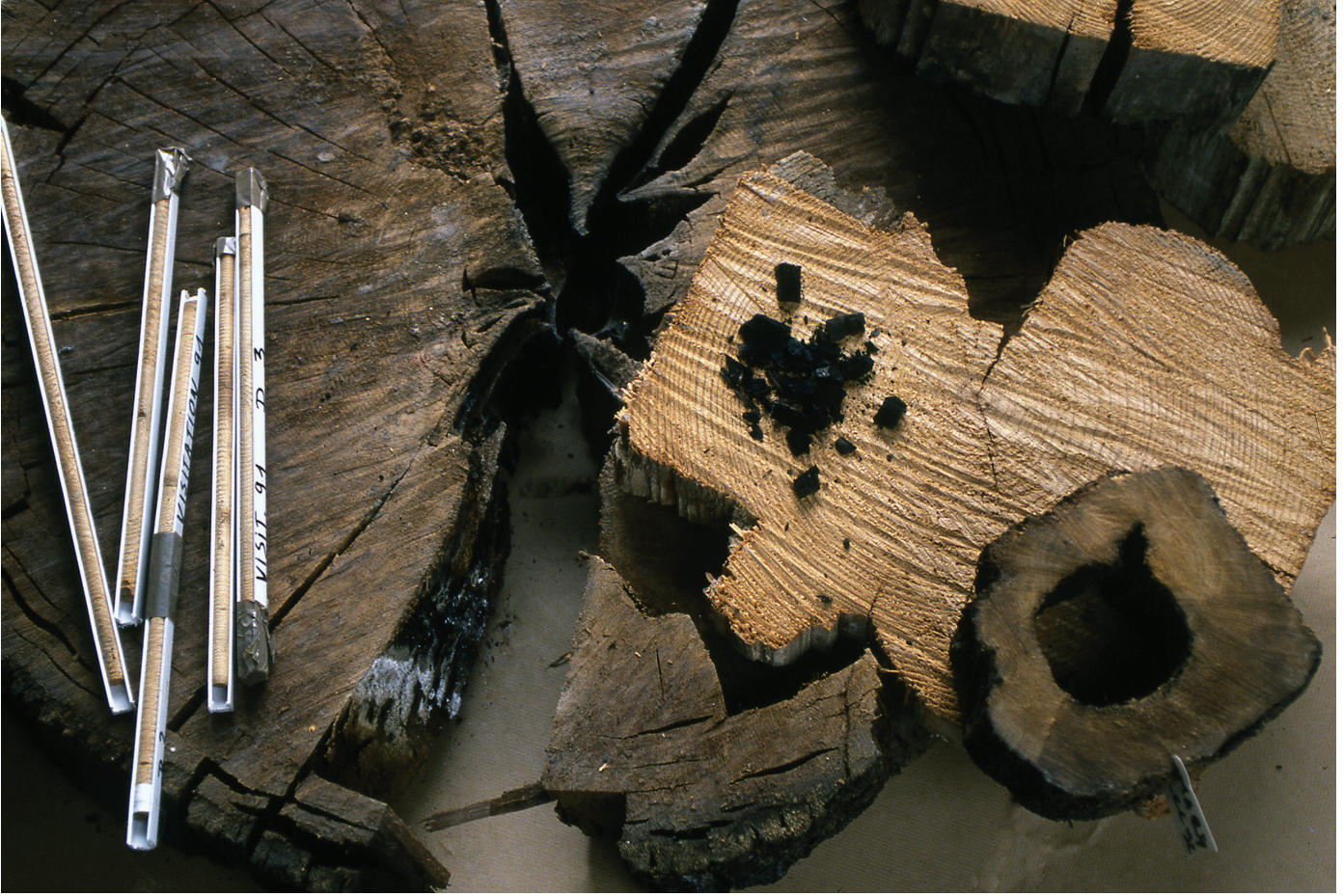
Equipment for sampling ancient wood for dendrochronology © Hervé Paitier, Inrap
