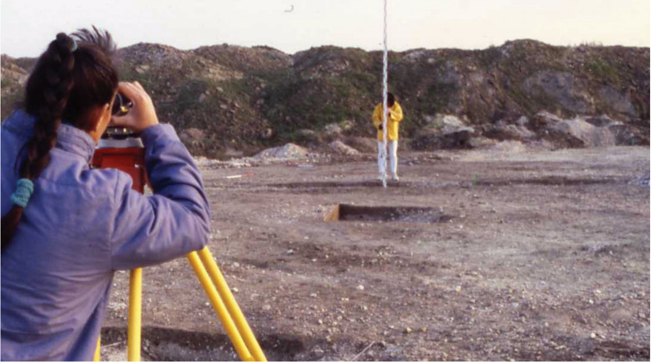
Recording the levels on the site of Fresnes-lès-Montauban, using a theodolite © Inrap
