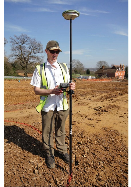
Surveying with GPS (Kent, England) © Canterbury Archaeological Trust
